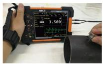
Thickness measurement on pipe
