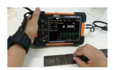
Thickness measurement on step block
