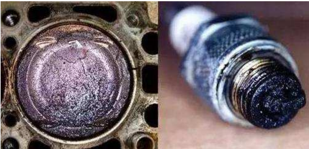
Piston and spark plug carbon
